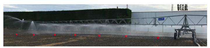
Bucket testing is a simple and costeffective way to ensure your irrigator is working efficiently.
